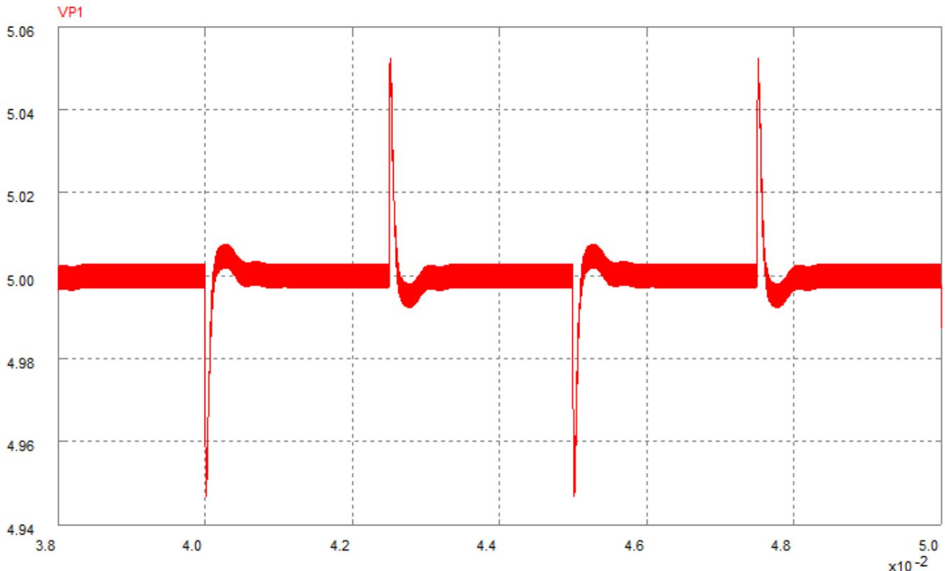
**Step input voltage response: 10 V -> 11 V -> 10 V**
