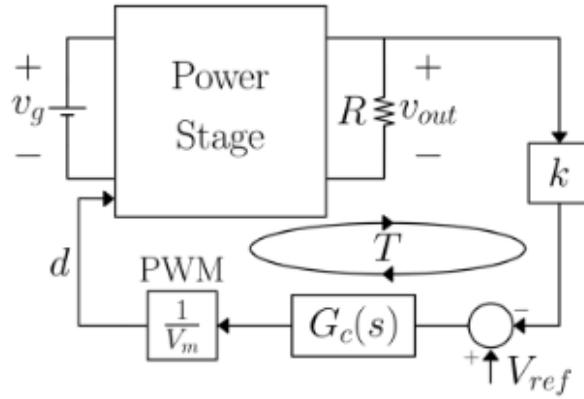
Block diagram of the voltage regulator system with a feedback loop  $T(s)$  consisting of the D4 converter power stage characterized by its control to output transfer function  $G_{vd} = \hat{v}_{out}/\hat{d}$ , resistive divider gain  $k$ , compensator transfer function  $G_c(s)$ , and PWM gain  $F_M = 1/V_M$ .
