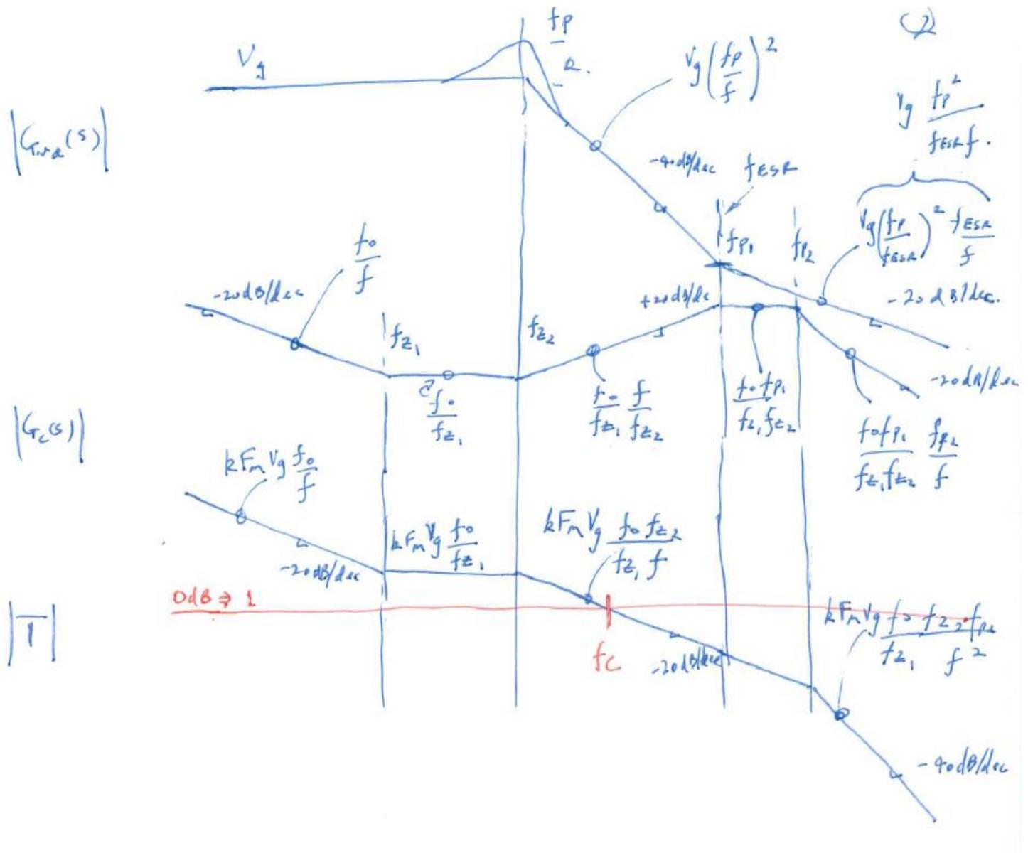
Compensator transfer function,  $G_c(s)$ , and resulting loop gain,  $T$ :
